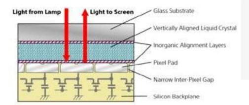
The LM8K panel in cross section. Light from the projection lamp enters through the glass substrate at the top, reflects off the mirrored surface and passes back out through the Liquid Crystal, toward the screen.
